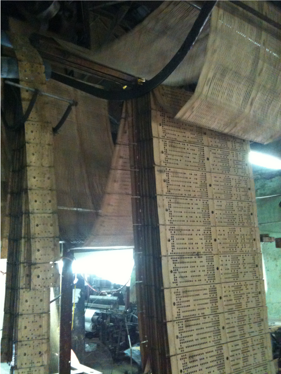
Figure 1: Punch cards used in a Jacquard silk loom at a workshop in Van Phuc silk village, Hanoi, Vietnam.
